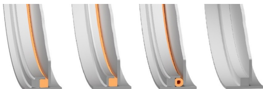
Example of seals from left: Figure 1 & 2: Fiberglass seal. Figure 3: Rubber gasket. Figure 4: Steel seal.
